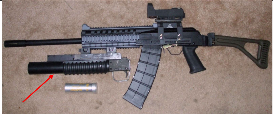
Pictured: Saiga 12 gauge semiautomatic shotgun with 37 mm flare launcher attached under the barrel. Grenade launcher will look similar.
